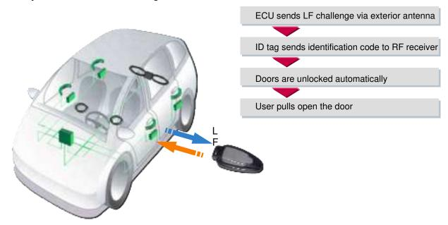
Figure 1: Principle of Communication
