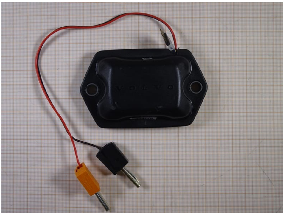
Photo 7: Modification for external power supply
