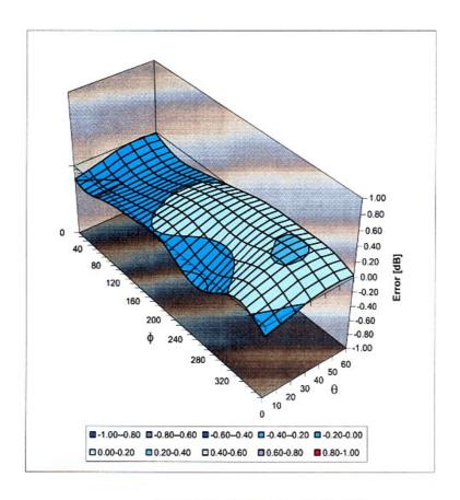
Spherical Isotropy Error < ± 0.4 dB
