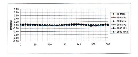
Axial Isotropy Error < ± 0.2 dB
