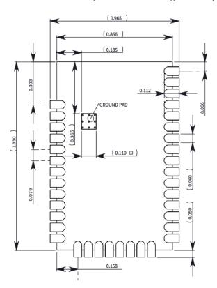
The recommended footprint includes an additional ground pad that you must solder to the corresponding pad on the XTC device. This ground pad transfers heat generated during transmit mode away from the
