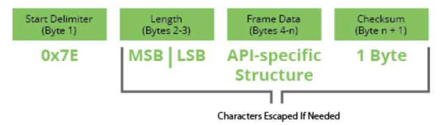
MSB = Most Significant Byte, LSB = Least Significant Byte
