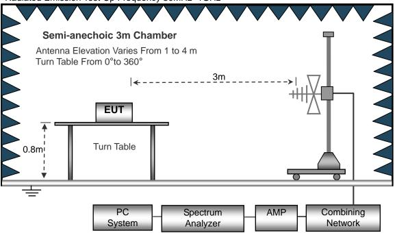
(C) Radiated Emission Test-Up Frequency Above 1GHz
