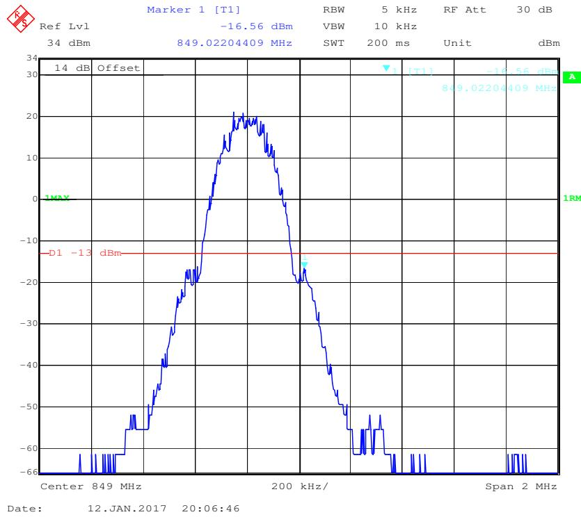
**PCS Band, Left Band Edge for GPRS Mode**
