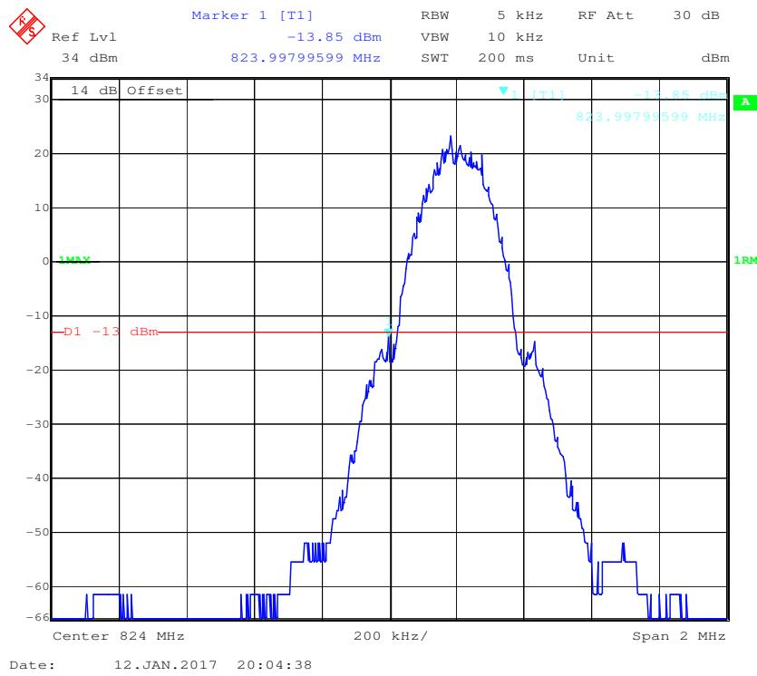
**Cellular Band, Right Band Edge for GPRS Mode**
