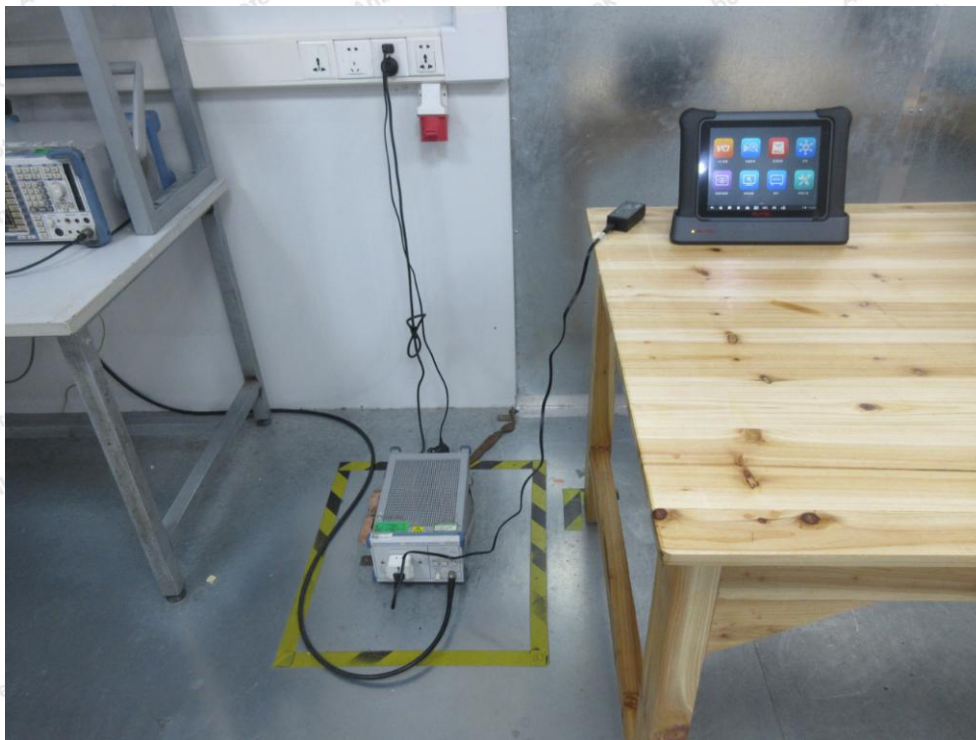
Photo of Conducted Emission Measurement
