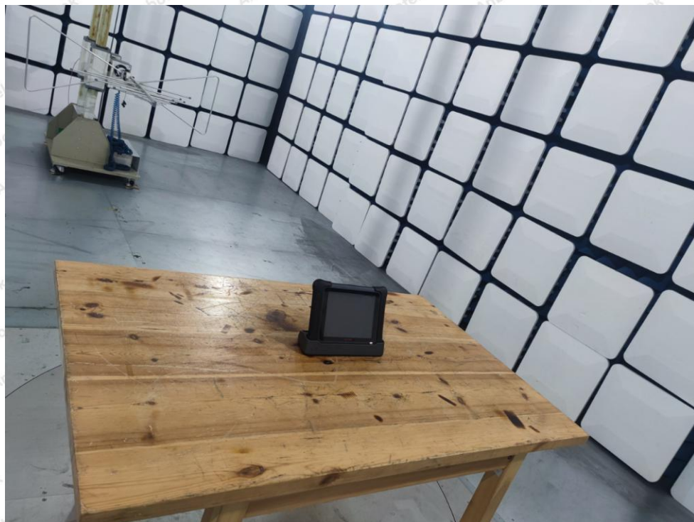
Photo of Radiation Emission Test
