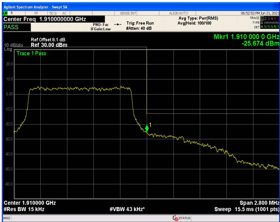
Band2 QAM16 BW=1.4MHz Channel=19193 RB Size=1 Position=#0
