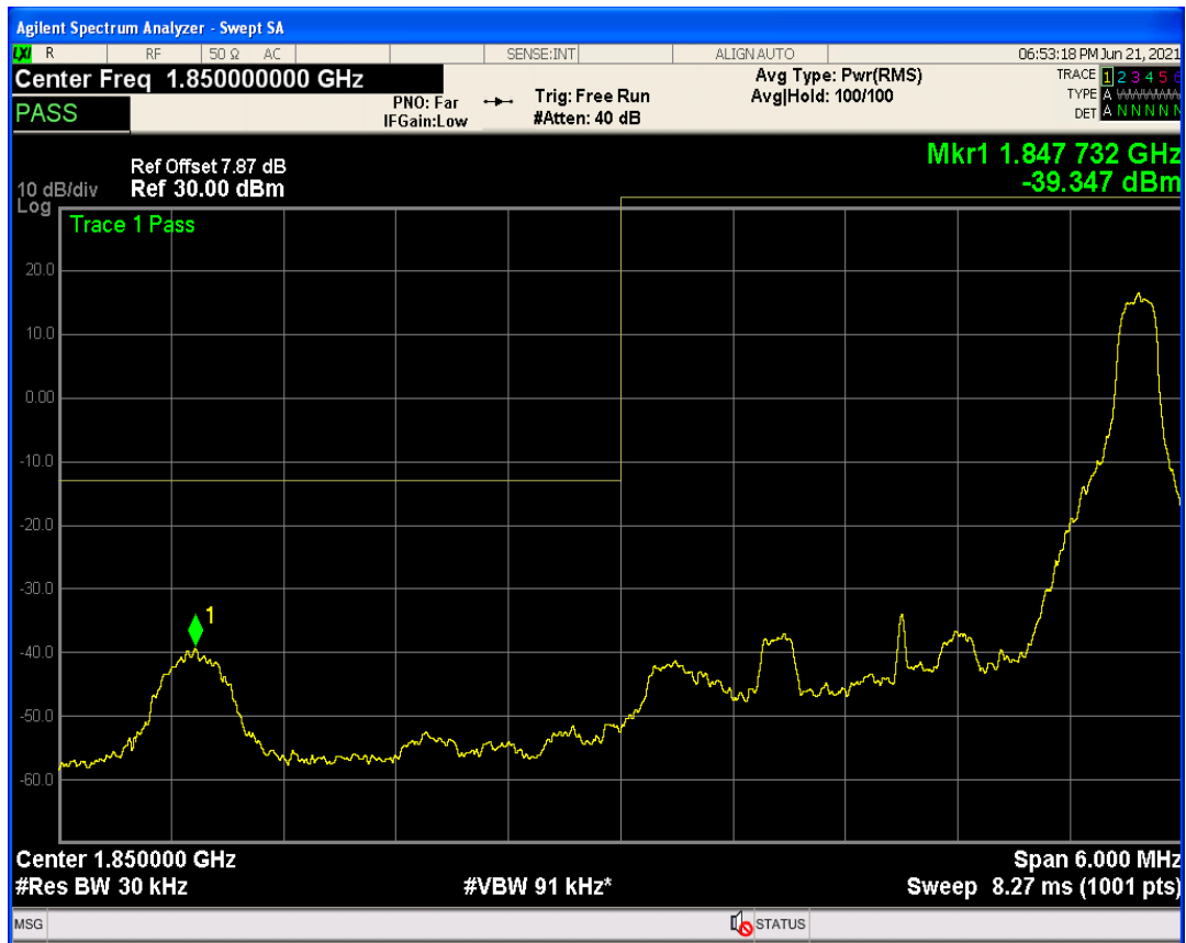
Band2 QPSK BW=3MHz Channel=18615 RB Size=15 Position=#0
