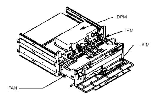
The EBC utilizes the DE as its external enclosure for environmental protection. four lifting eyes are provided at the top of the EBC for installation at the cell site.
