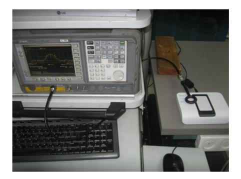
Photograph No.8 Setup for band edge emission measurements (DTS part)
