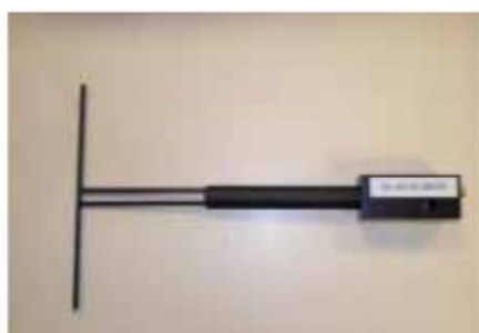
Figure 1 – Satimo COMOSAR Validation Dipole
