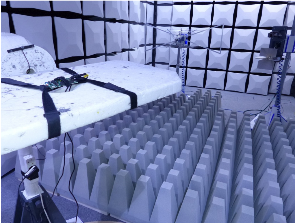
Photo 5: Test setup for radiated measurements above 1 GHz
