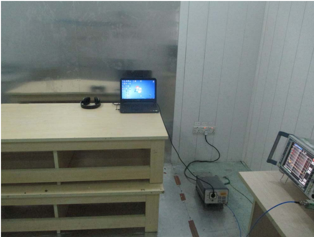
FCC RADIATED EMISSION TEST SETUP
