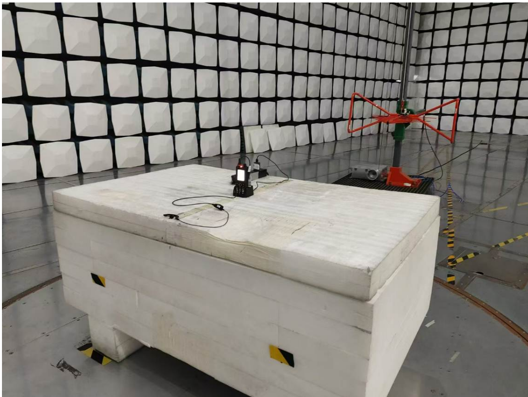
Radiated Emission 30M-1GHz View
