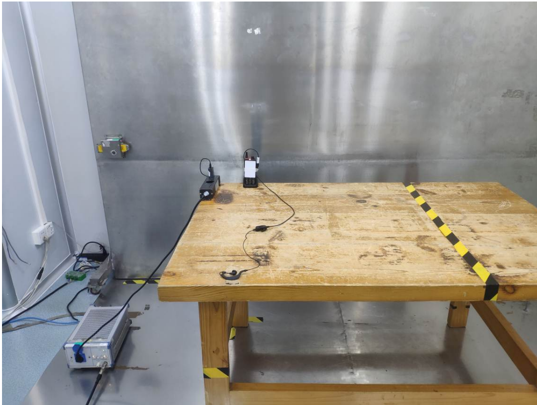
Conducted Emissions Side View
