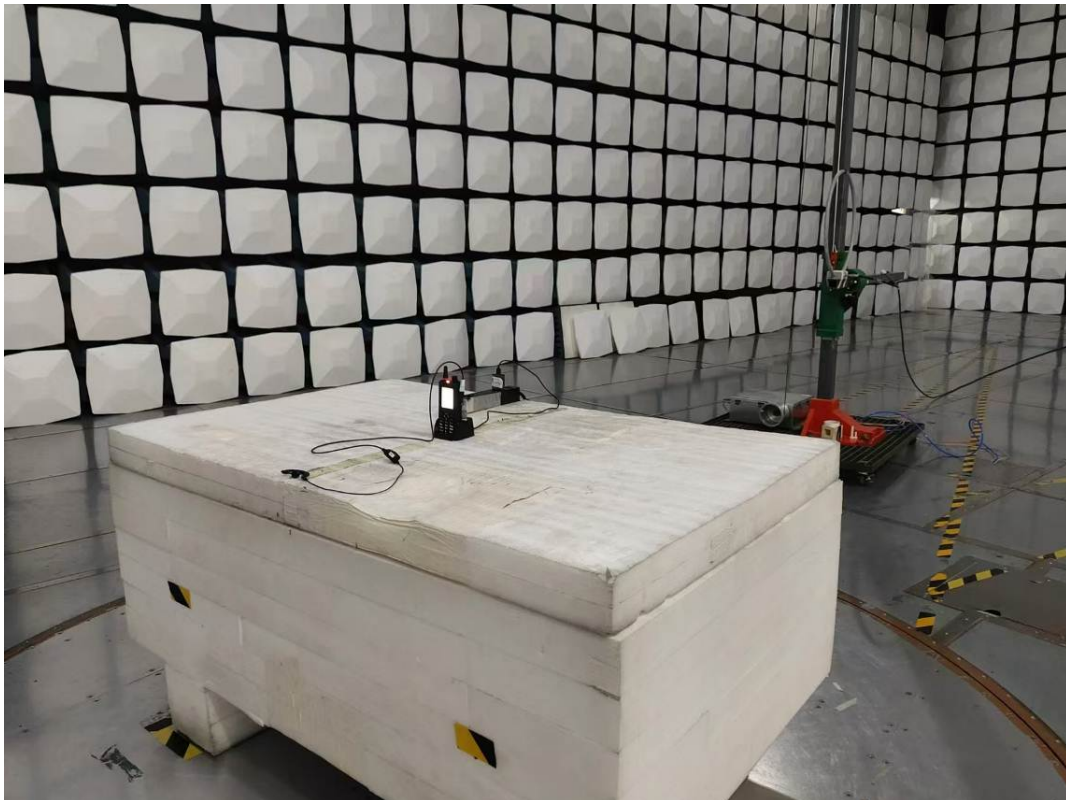
Radiated Emission 9k-30MHz Perpendicular View
