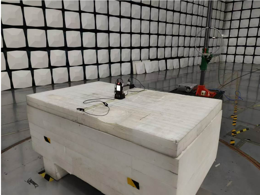
Radiated Emission 9k-30MHz Perpendicular View
