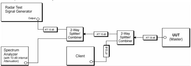
(Example Conducted Setup where UUT is a Master and Radar Test Waveforms are injected into the Master)
