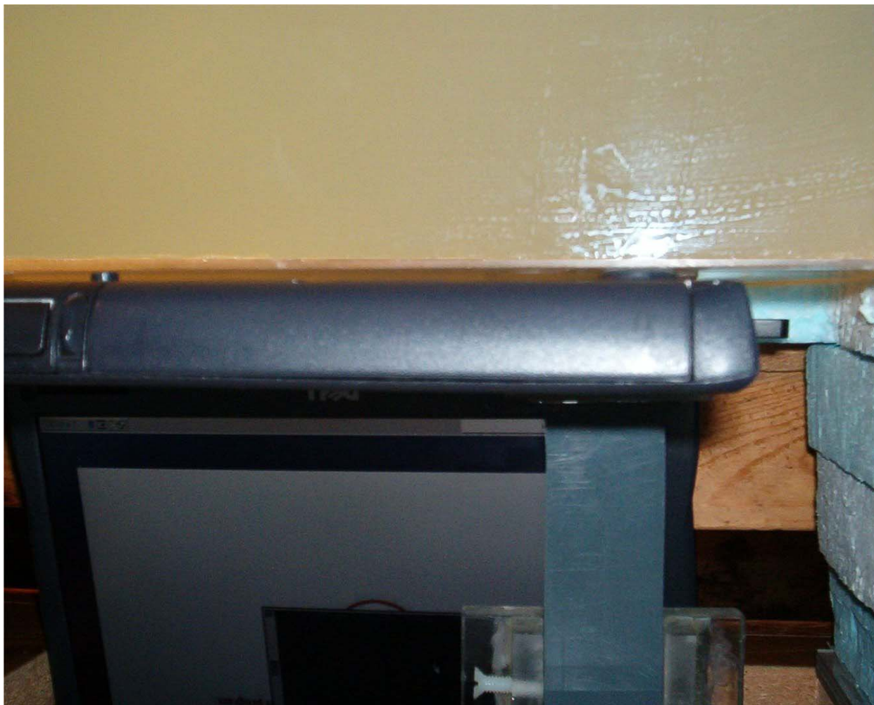
Fig. 2. Photograph of the bottom of the Dell Model PP01L Host Computer with Arcadyan EZ-Stream Universal Wireless Cardbus Adapter pressed against the bottom of the planar phantom. This Configuration 1 – Laptop position for SAR testing .
