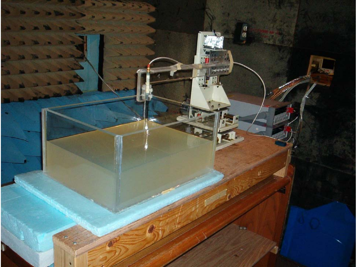
Fig. 4. Photograph of the three-dimensional stepper-motor-controlled SAR measurement system using a planar phantom.
