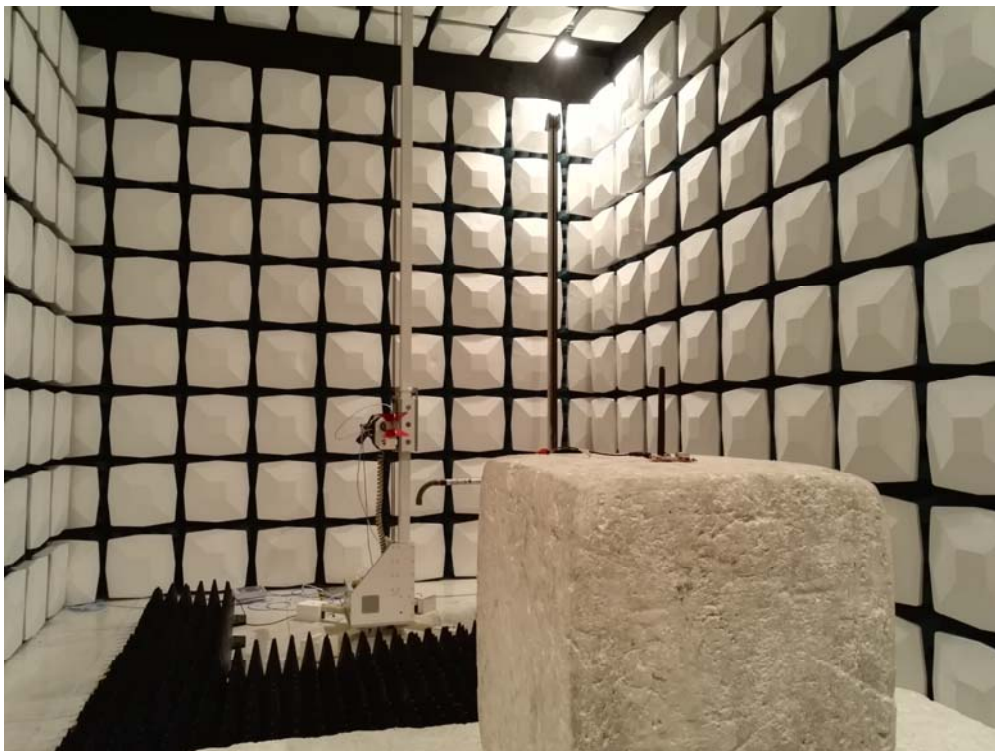
Description: EIRP Test Setup
