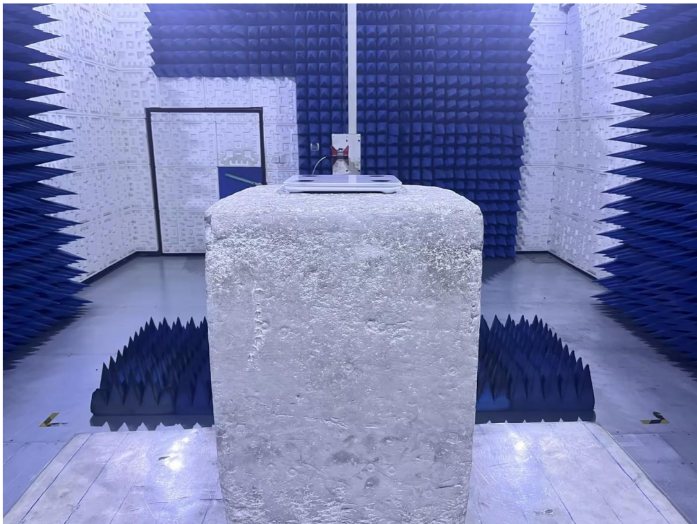
RADIATED EMISSION TEST SETUP ABOVE 1GHz
