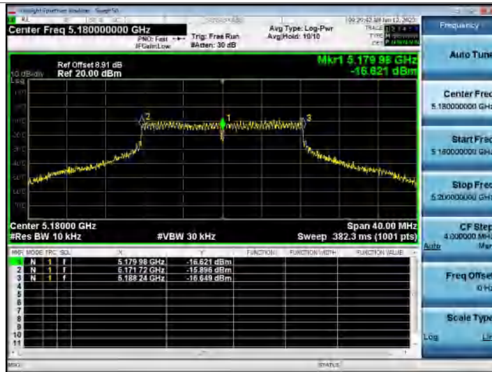
Freq. Stability 0C 120V a 5180MHz Ant1 0 Minutes
