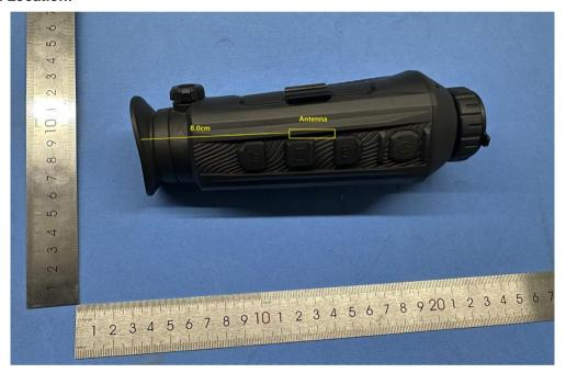
Minimum distance from antenna to eyepiece (Head): 8cm Minimum distance from antenna to casing (Extremity): 0.5cm
