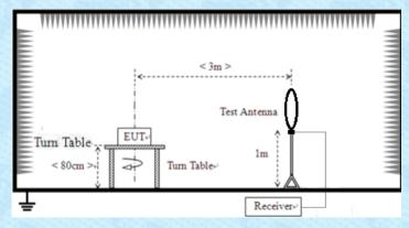
For radiated emissions from 30MHz to1GHz
