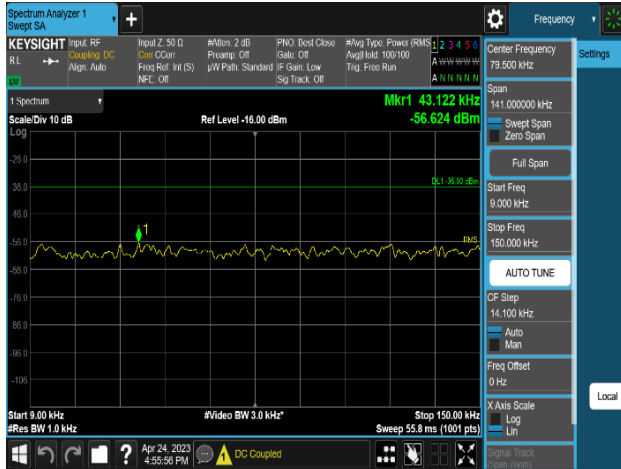
Plot 8-441. Conducted Spurious Emission Plot 9 kHz to 150 kHz
