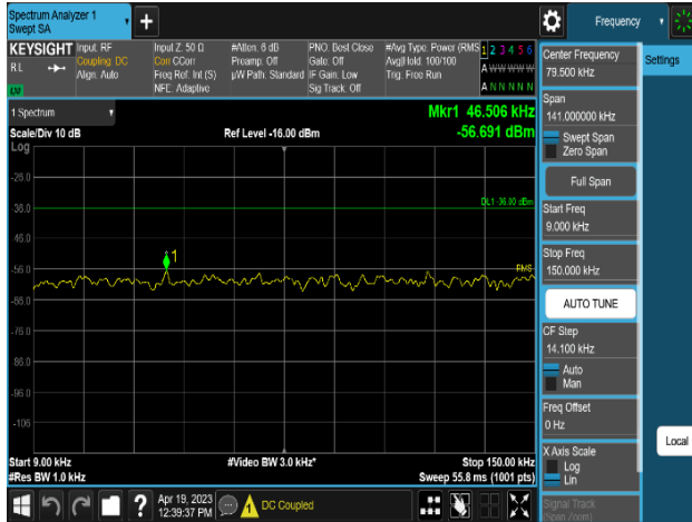
Plot 8-483. Conducted Spurious Emission Plot 9 kHz to 150 kHz (NR n5_2C_5M+5M_2T_16QAM - High Channel, Port 0)
