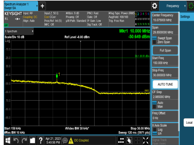
Plot 8-460. Conducted Spurious Emission Plot 150 kHz to 30 MHz (DSS B(n)5_2C_10M+10M_2T_16QAM - High Channel, Port 0)
