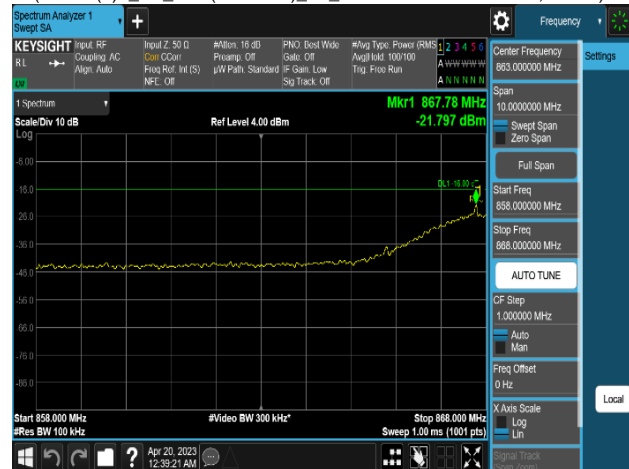
Plot 8-456. Conducted Spurious Emission Plot 858 MHz to 868 MHz (DSS B(n)5_1C_10M(5:5 Ratio)_2T_256QAM - Low Channel, Port 1)
