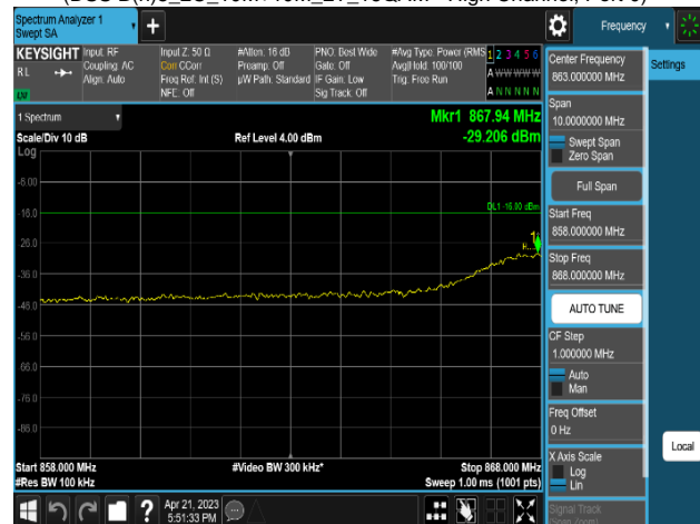
Plot 8-462. Conducted Spurious Emission Plot 858 MHz to 868 MHz (DSS B(n)5_2C_10M+10M_2T_16QAM - High Channel, Port 0)
