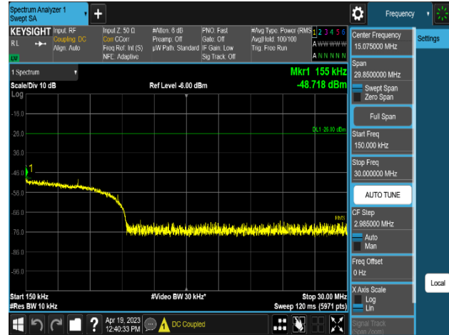
Plot 8-484. Conducted Spurious Emission Plot 150 kHz to 30 MHz (NR n5_2C_5M+5M_2T_16QAM - High Channel, Port 0)
