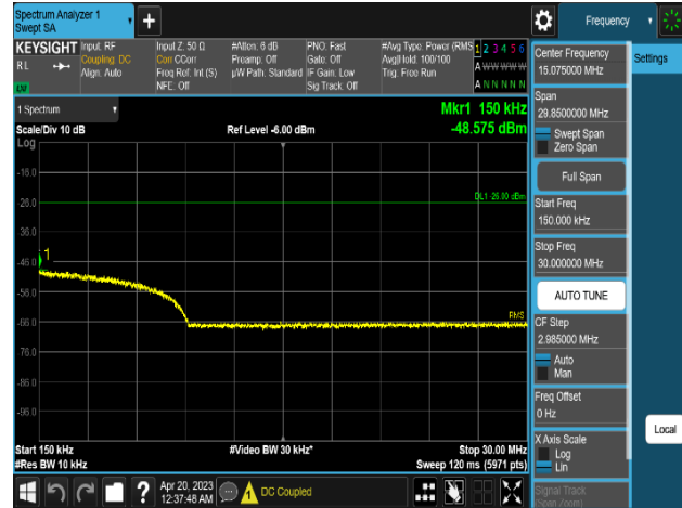
Plot 8-454. Conducted Spurious Emission Plot 150 kHz to 30 MHz (DSS B(n)5_1C_10M(5:5 Ratio)_2T_256QAM - Low Channel, Port 1)
