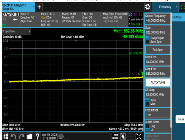
Plot 8-491. Conducted Spurious Emission Plot 30 MHz to 858 MHz (NR n5_2C_10M+15M_2T_16QAM - Middle Channel, Port 0)
