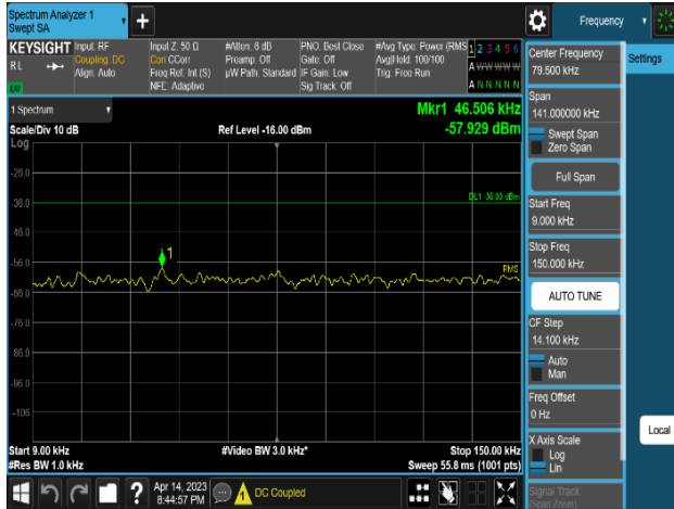
Plot 8-465. Conducted Spurious Emission Plot 9 kHz to 150 kHz (NR n5_1C_5M_2T_QPSK - Low Channel, Port 0)
