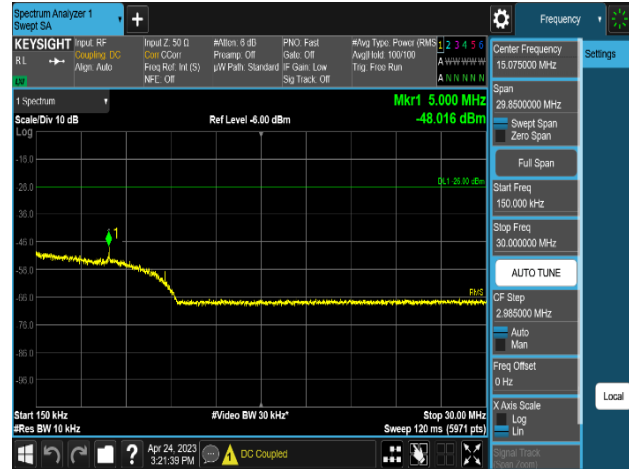
Plot 8-436. Conducted Spurious Emission Plot 150 kHz to 30 MHz (LTE B5_2C_5M+5M_2T_16QAM - High Channel, Port 0)
