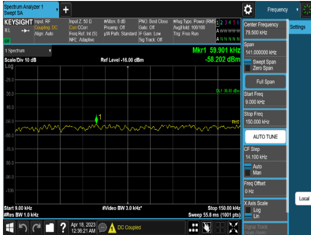
Plot 8-471. Conducted Spurious Emission Plot 9 kHz to 150 kHz (NR_n5_1C_10M_2T_256QAM - High Channel, Port 0)
