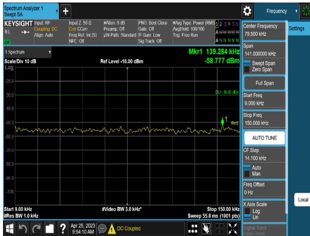
Plot 8-501. Conducted Spurious Emission Plot 9 kHz to 150 kHz (MSR 2C_DSS B(n)5_1C_10M+LTE B5_1C_5M_2T_QPSK - High Channel, Port 0)
