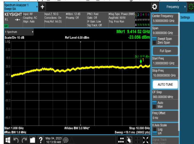
Plot 8-464. Conducted Spurious Emission Plot 1 GHz to 10 GHz (DSS B(n)5_2C_10M+10M_2T_16QAM - High Channel, Port 0)
