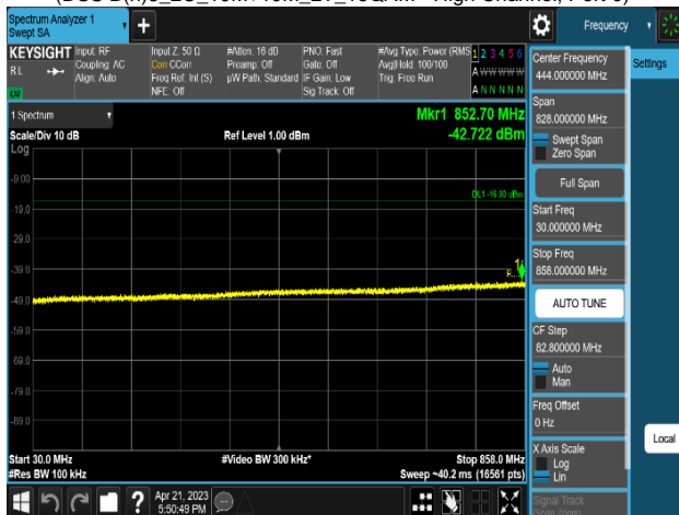
Plot 8-461. Conducted Spurious Emission Plot 30 MHz to 858 MHz (DSS B(n)5_2C_10M+10M_2T_16QAM - High Channel, Port 0)
