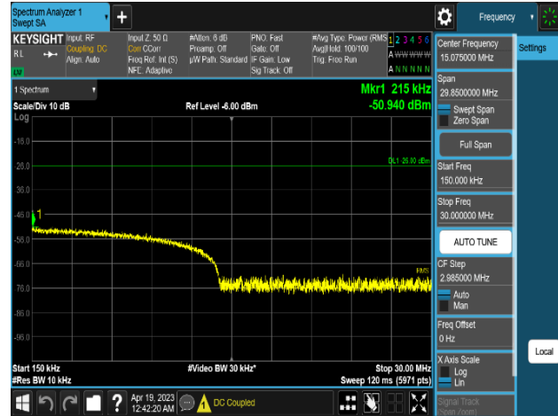
Plot 8-478. Conducted Spurious Emission Plot 150 kHz to 30 MHz (NR n5_1C_15M_2T_64QAM - Low Channel, Port 0)
