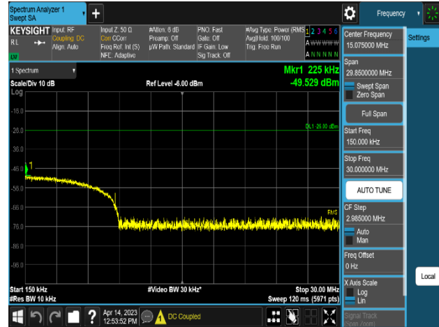
Plot 8-430. Conducted Spurious Emission Plot 150 kHz to 30 MHz (LTE B5_1C_10M_2T_16QAM - High Channel, Port 0)
