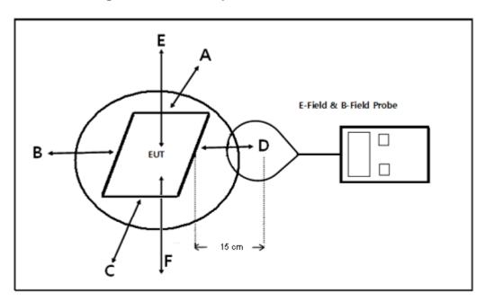
Note: Due to installation limitations no tests from the underside of the charging device (Test Position F) are required.
