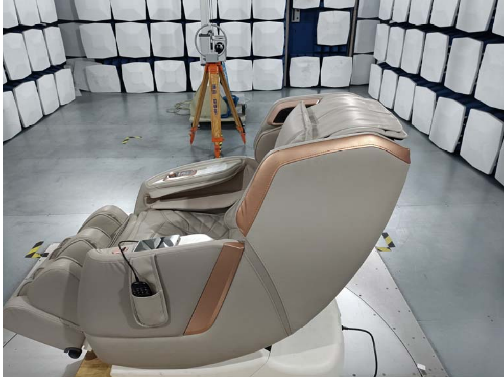
Radiated Emission Test Setup:
