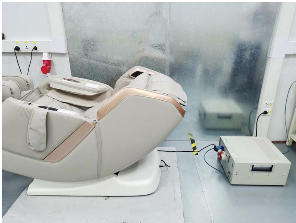
Conducted Emission Test Setup:
