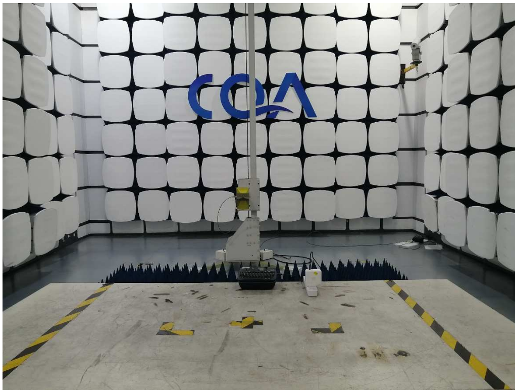
Photograph 3: Set-up for Radiated Emission, above 1GHz
