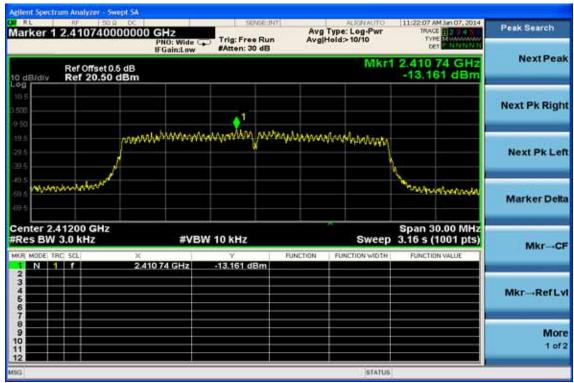
**Power Spectral Density Test Plot (CH-Mid)**
