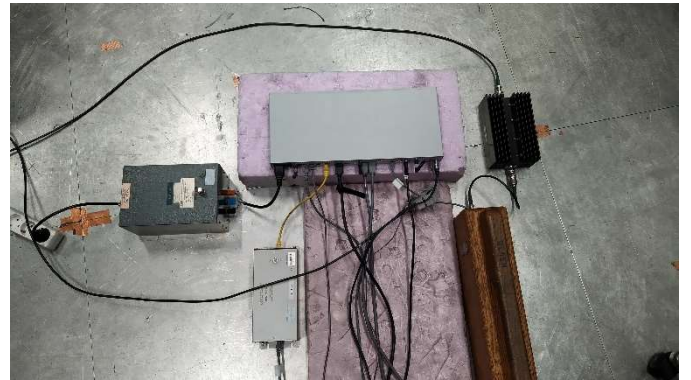
Test set-up for Conducted RF disturbance immunity (Signal ports)
