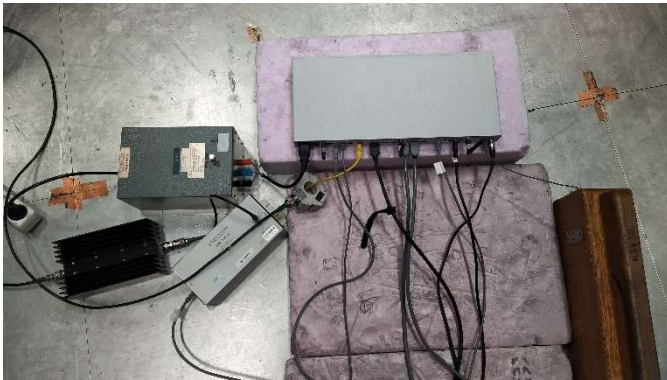
Test set-up for Conducted RF disturbance immunity (LAN/PoE-port)
