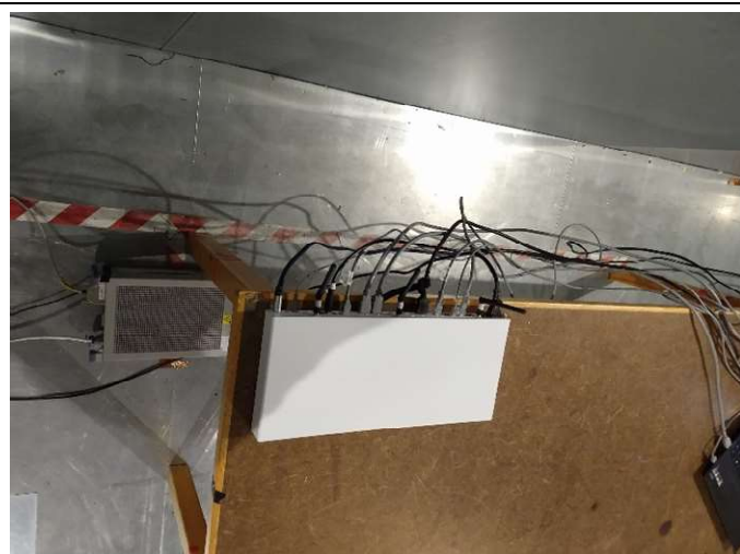
Test set-up for Conducted emissions measurements (AC mains)
