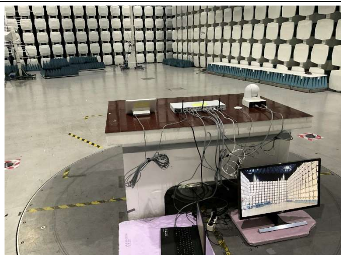
Test set-up for Radiated emissions measurements (Below 1GHz, FCC)
