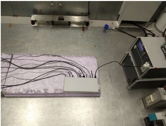
Test set-up for Electric fast transients, Surge and Voltage dips and interruptions immunity (AC mains)
