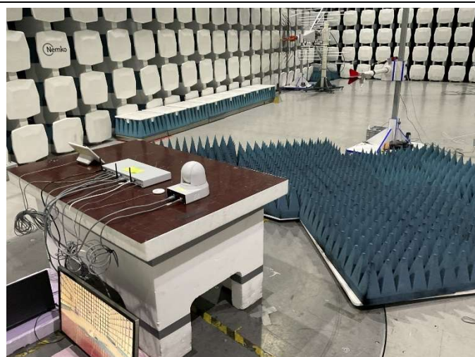
Test set-up for Radiated emissions measurements (Above 1 GHz, FCC)
