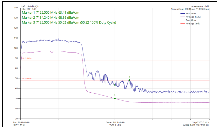
Figure 77 - 802.11ax, HE40, SU, TxBF, Core 0-1 - 7085 MHz, Band Edge Frequency 7125 MHz
