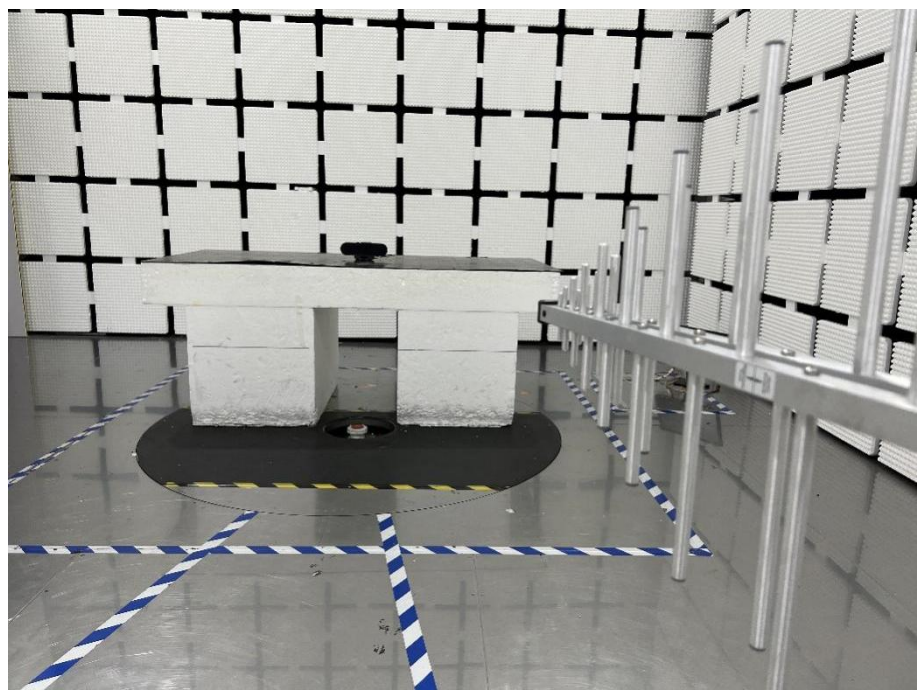
Radiation Emission Test Setup (30MHz to 1GHz)
