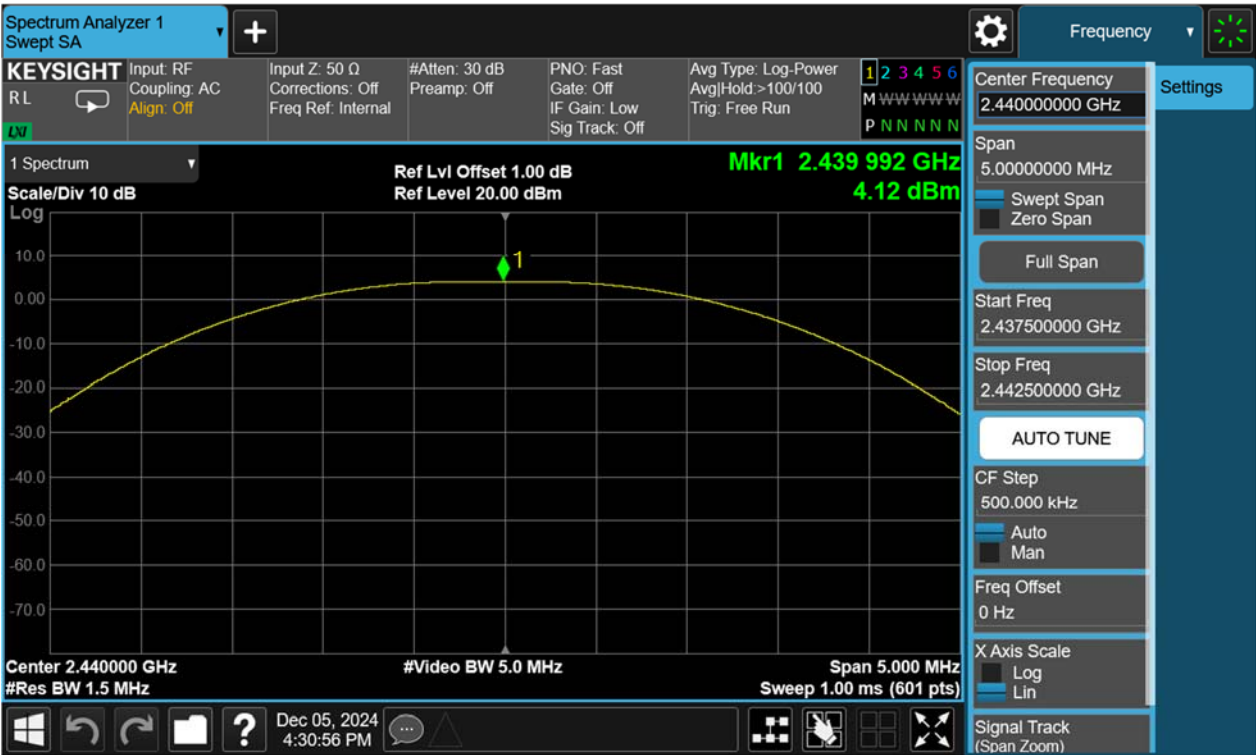
Figure 2: Peak Output Power, 2440MHz, BLE-1Mbps
