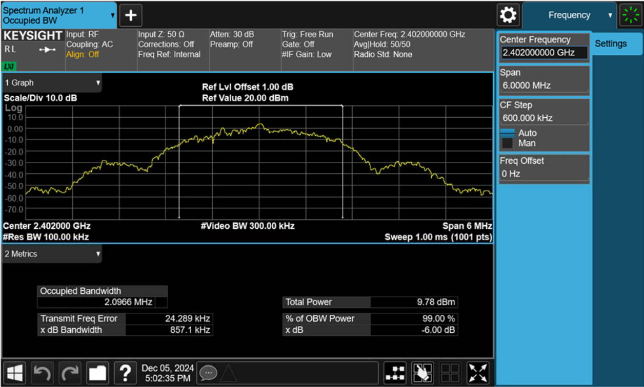
Figure 10: 6dB Bandwidth, 2402MHz, BLE-2Mbps
