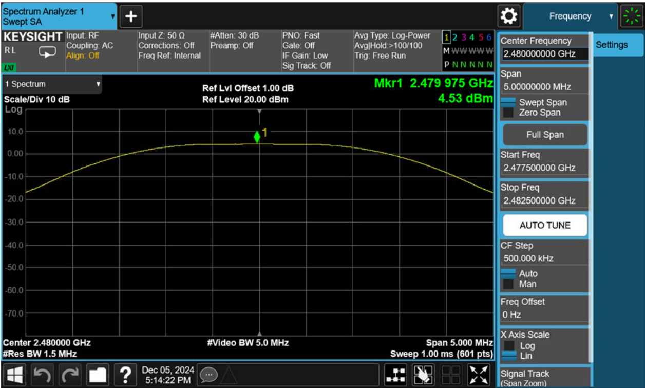
Figure 6: Peak Output Power, 2480MHz, BLE-2Mbps
