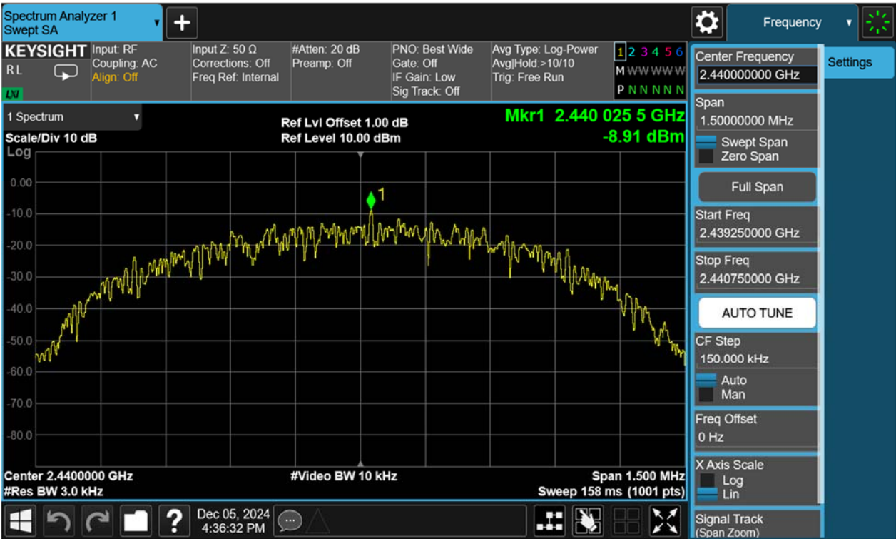
Figure 14: Power Spectral Density, 2440MHz, BLE-1Mbps
