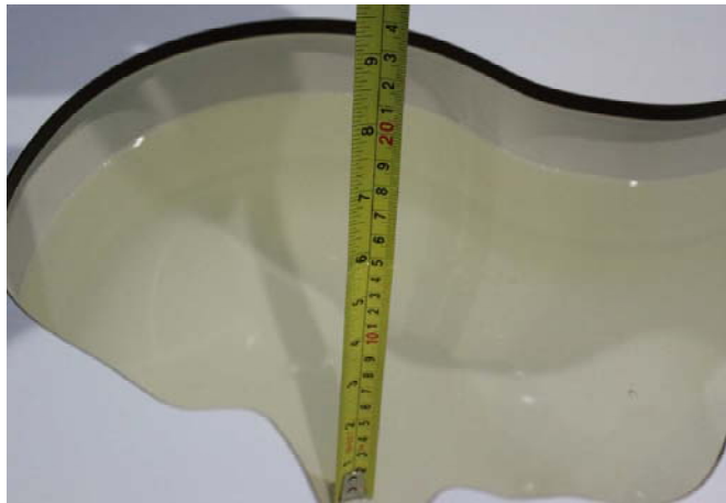
Liquid depth in the head phantom (5GHz)
