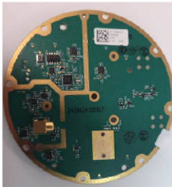
Yahsat T-TAC Vehicular Antenna PCBA BottomView
