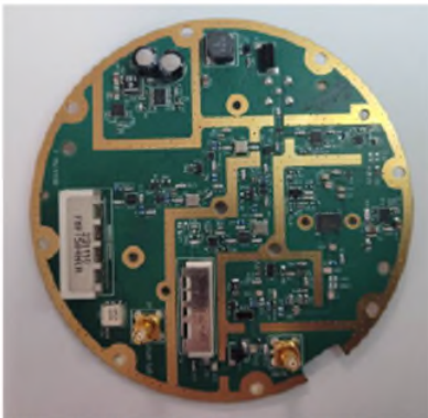
Yahsat T-TAC Vehicular Antenna PCBA TopView
