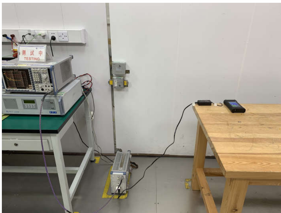
Conducted Emissions Test Setup
