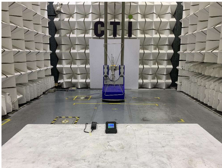
Radiated spurious emission Test Setup-1(Below 1GHz)
