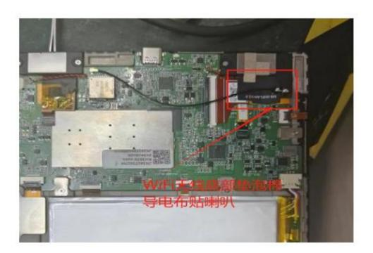
8. Schematic diagram of antenna assembly
