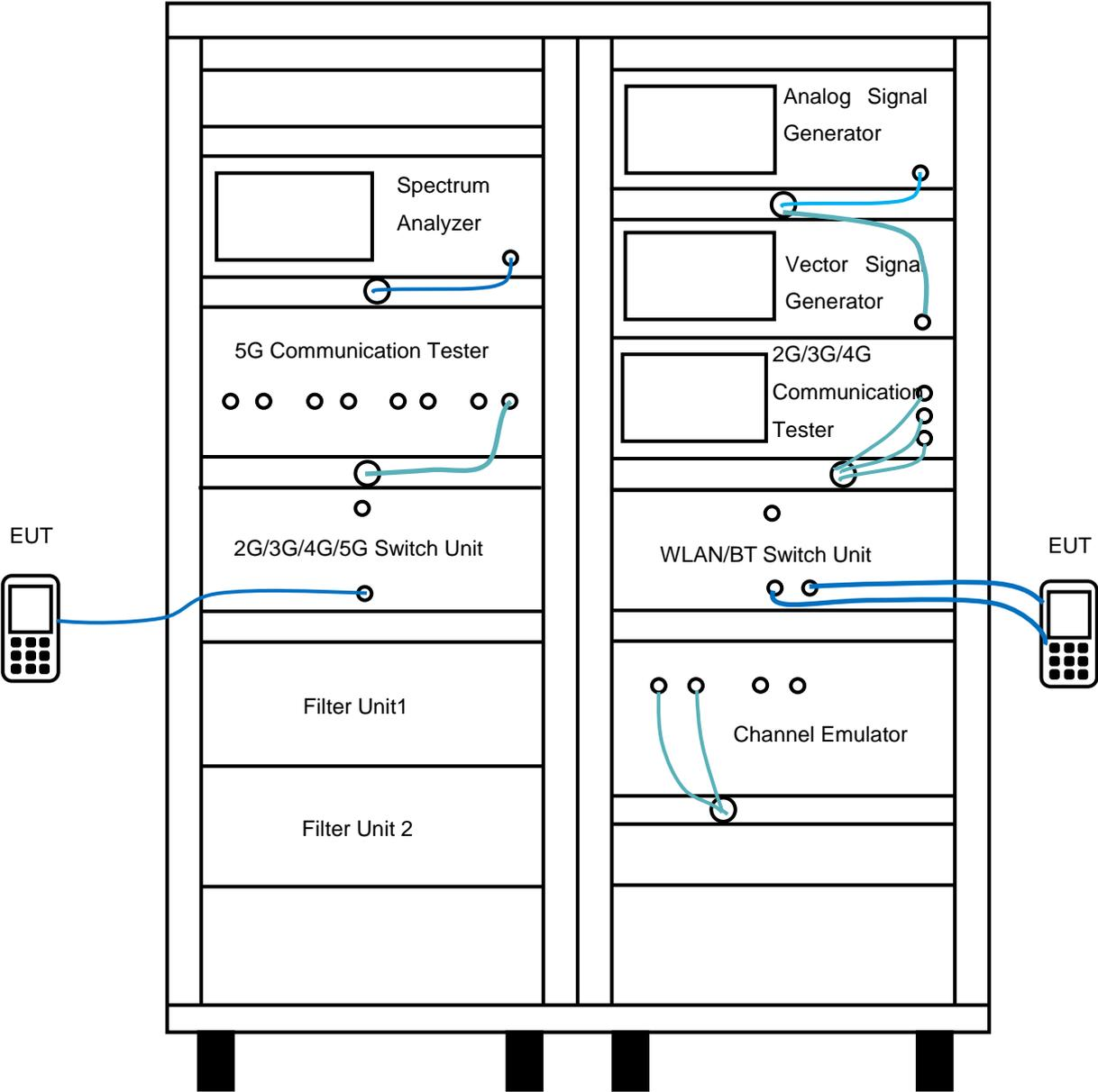
Diagram of Measurement Configuration for Radiation Test
