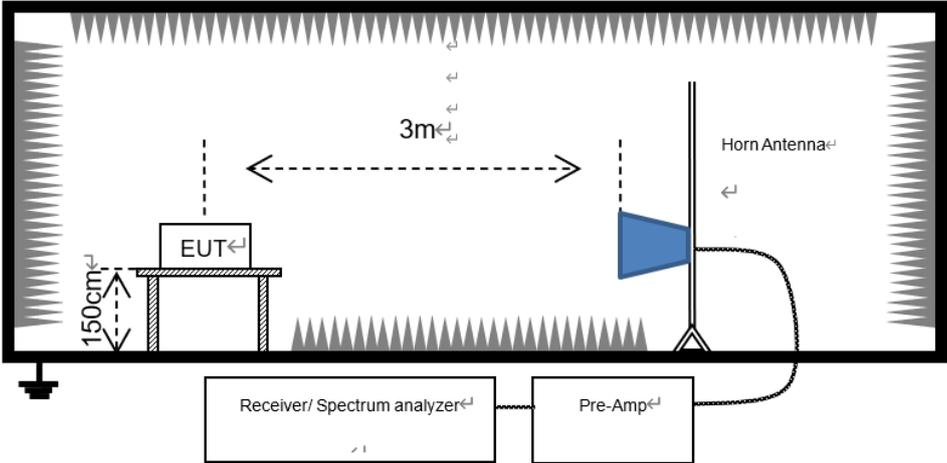
Note: Measurements below 1GHz are done with a table height of 0.8m and above 1GHz are done with a table height of 1.5m. In addition, there is RF absorbing material on the floor of the test site for above 1GHz measurement.
