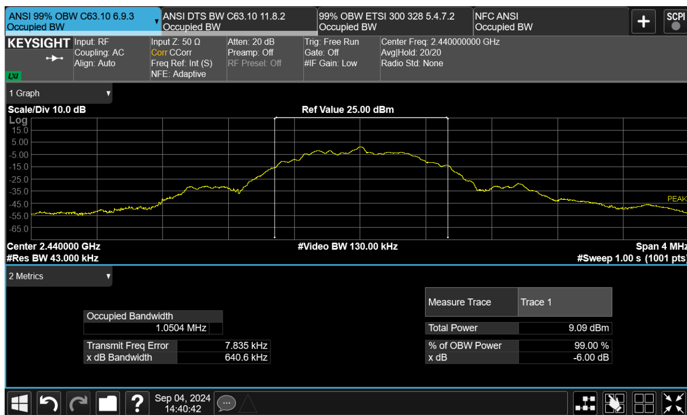
Figure TR10.2: Occupied bandwidth data for BLE 1 Mbps at mid channel (2440 MHz)
