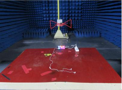
RADIATED EMISSION TEST (Frequency above 1GHz)
