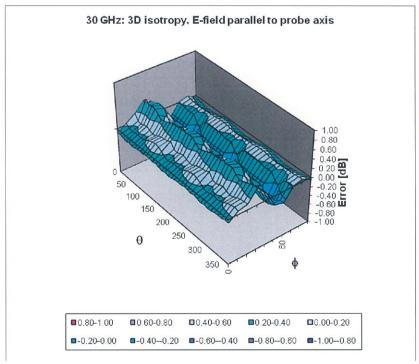
Probe isotropy for E<sub>tot</sub>: probe rotated  $\phi$  = 0° to 360°, tilted from field propagation direction  $\vec{k}$  Parallel to the field propagation ( $\psi$  =0° - 90°): deviation within ± 0.49 dB Normal to field orientation ( $\theta$  =0° - 90°): deviation within ± 0.56 dB
