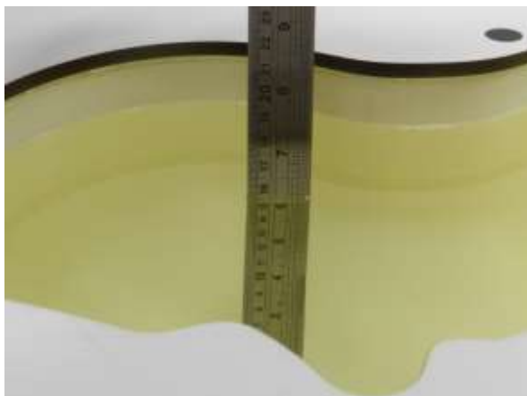
Fig 11.1 Photo of Liquid Height for Head SAR
