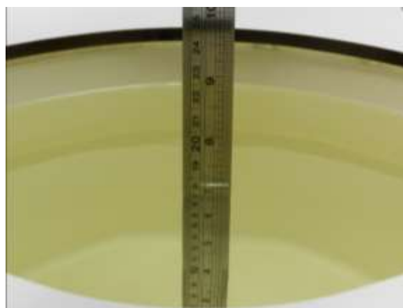
Fig 11.2 Photo of Liquid Height for Body SAR
