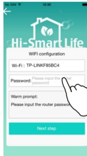
2. "Wi-Fi" shown in above picture is the wireless router the phone connected to. Users need to type in router password for binding. Then click "Next".
