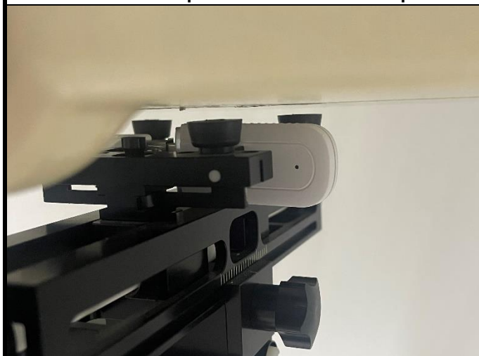
Vertical-Front of EUT with 0.5 cm Gap
