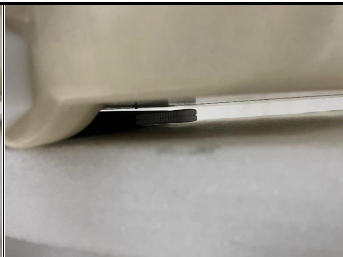
Horizontal-Down of EUT with 0.5 cm Gap
