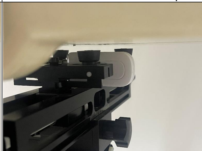
Vertical-Back of EUT with 0.5 cm Gap
