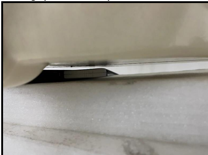
Horizontal-Up of EUT with 0.5 cm Gap
