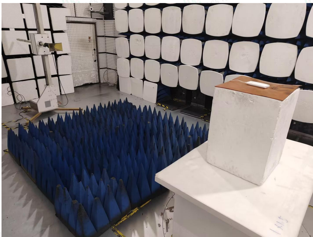
Radiated Emissions Measurement (Above 1GHz)
