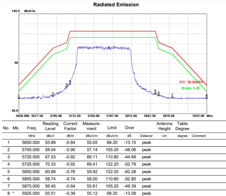
Note: For radiated Emissions from 18-40GHz, it is only the floor noise and less than the limit for more than 20dB. No necessary to take down.
