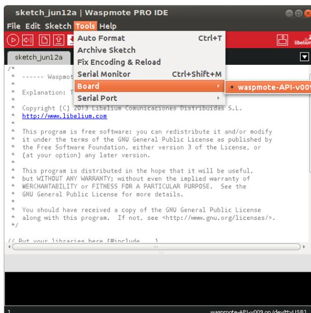
Figure : Selecting API for Waspmate Plug & Sense!
