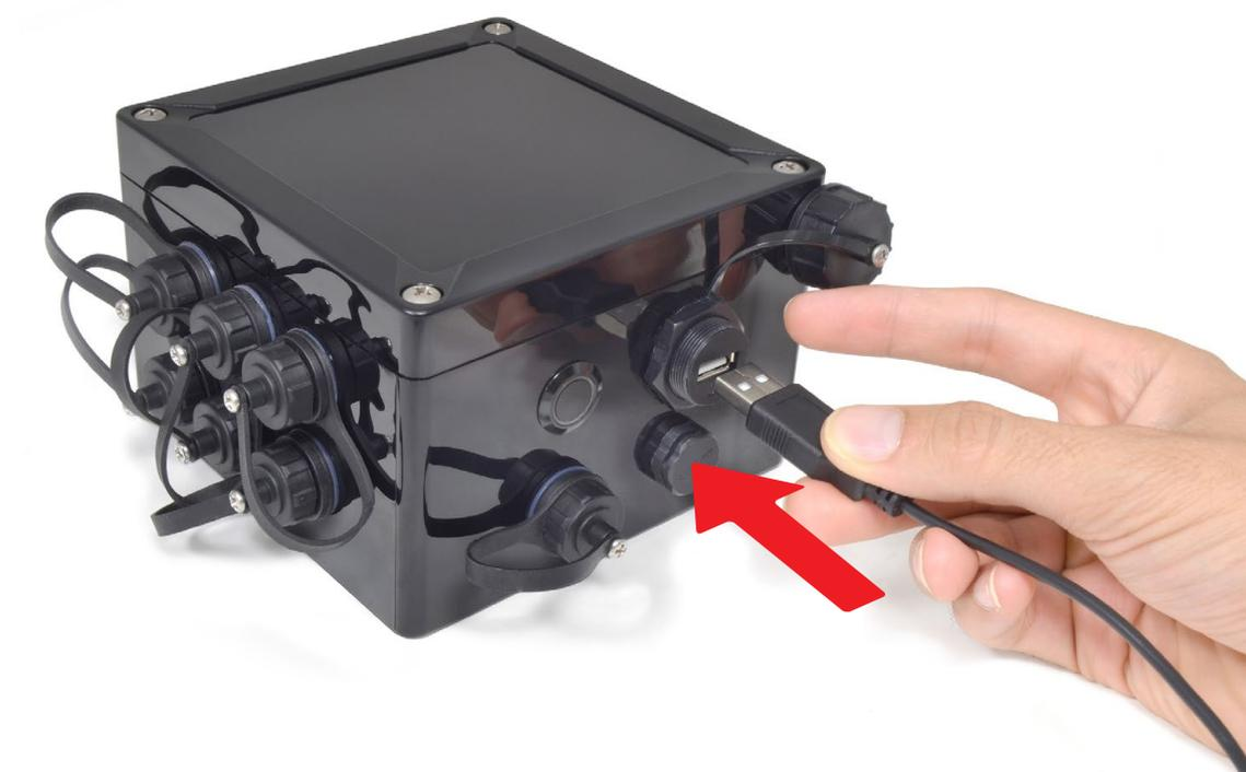
*Figure : Connecting the USB cable to Waspote*
