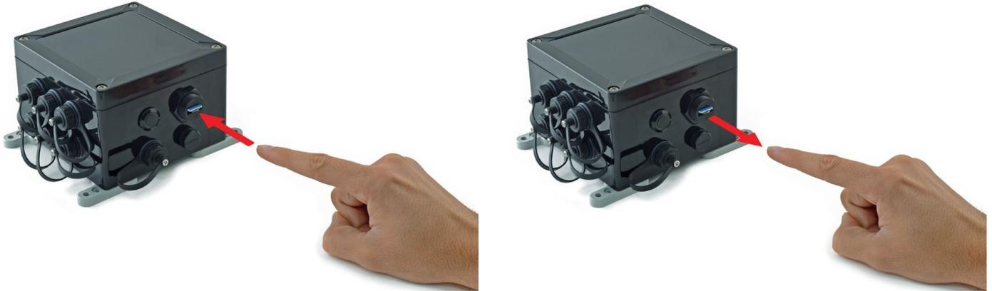
*Figure : Push-pull mechanism in the External SIM socket*
