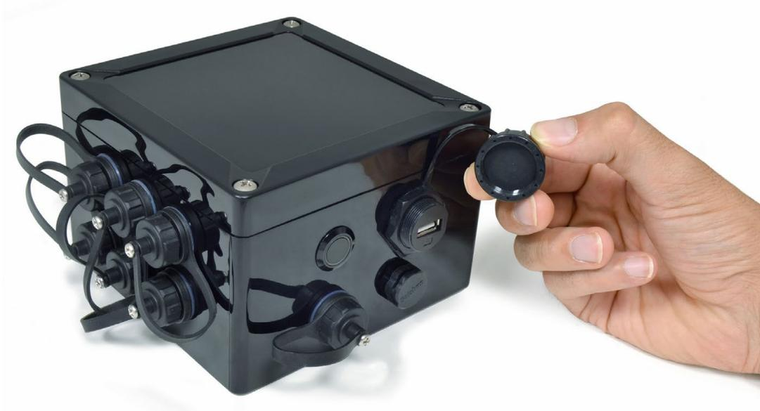
Figure : Removing the USB cap
