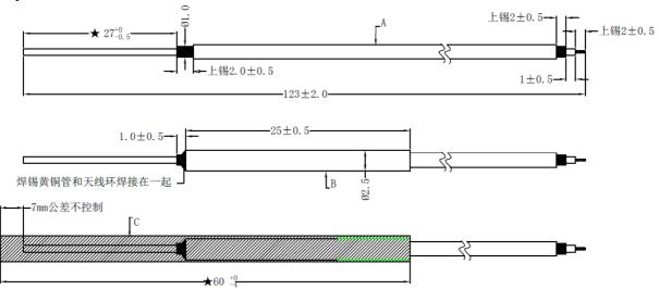
Figure 1 Physical dimension (mm)
