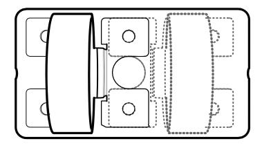
Use the included remote mounting plate to perform a custom, flush installation of the remote. Be careful not to drill into wiring or vehicle mechanisms. You are solely responsible for safely and securely mounting the unit and remote. Use the cut-out template below to assist in the installation.
