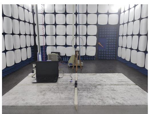
3. Radiated emission (9KHz-30MHz)
