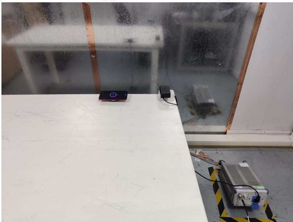
Conducted Emission-AC adapter charge mode
