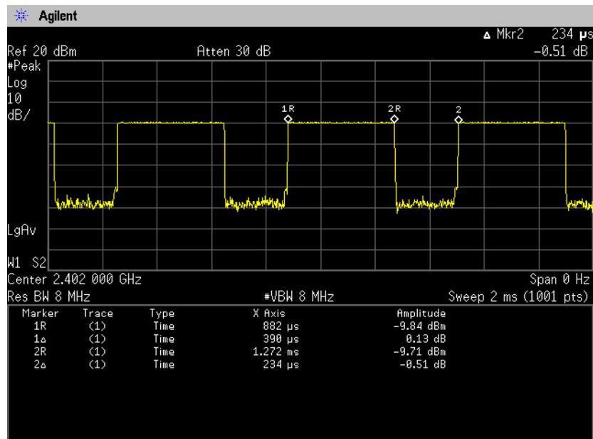
$$\text{Duty Cycle} = T_{\text{on}} / (T_{\text{on}} + T_{\text{off}}) = 390[\mu\text{s}] / (390[\mu\text{s}] + 234[\mu\text{s}]) = 62.5[\%]$$
