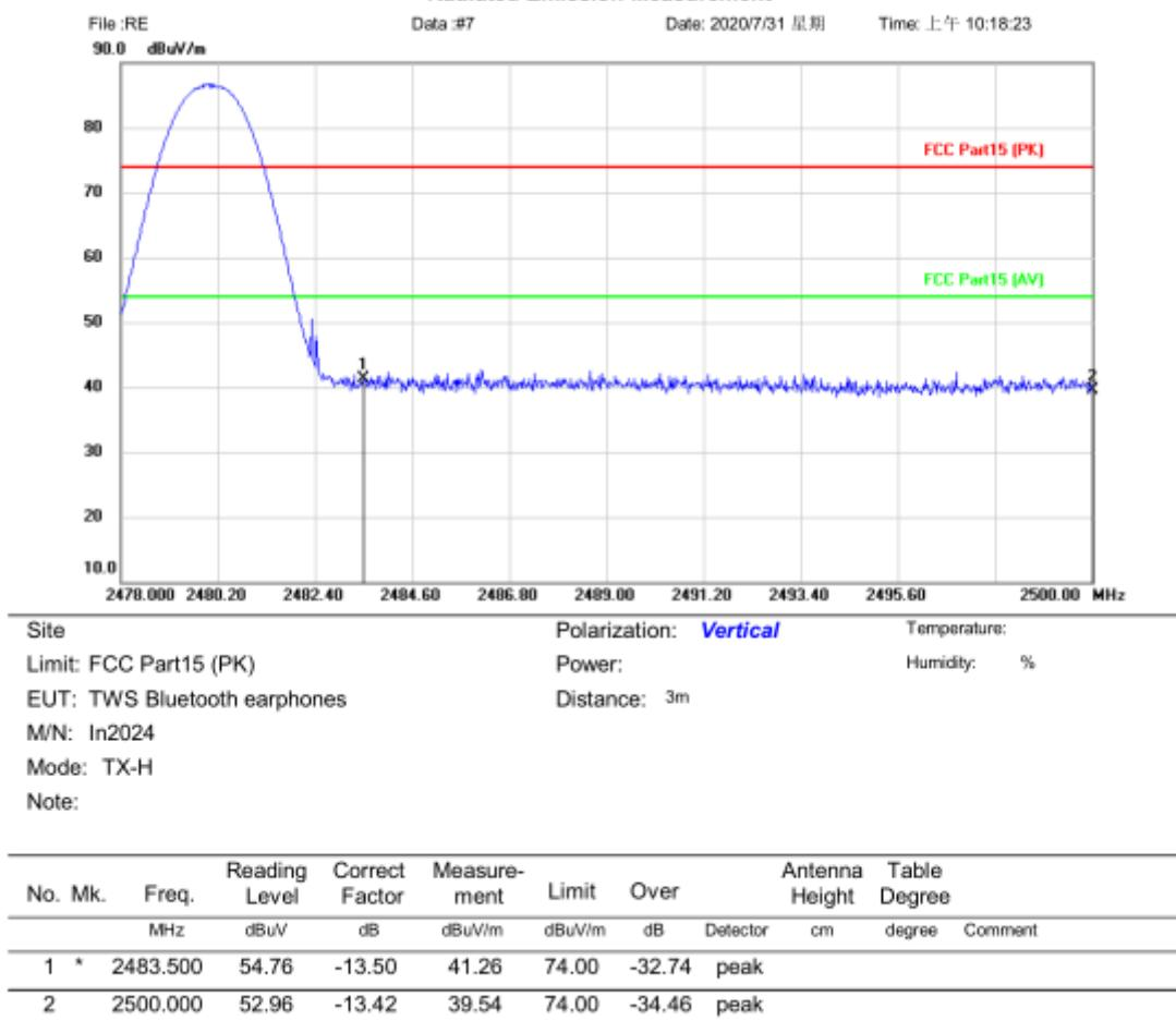
**Radiated Emission Measurement**
